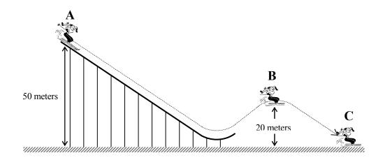
Assuming that the ramp is frictionless, use the principle of conservation of energy to find the speed of the skier at point  $\mathbf{B}$ . (This is the point where she reaches the maximum height in flight).
